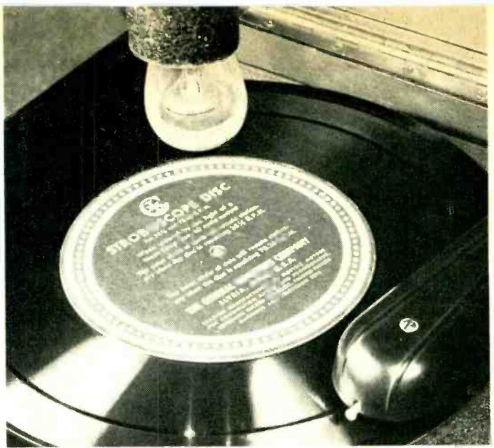
Set-up for checking speed of phonograph turntable with neon tube and stroboscope disc. Pickup is run through outside of record to establish normal load.
