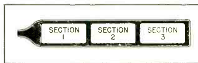
Fig. 3. Section 2 is more apt to fail, due to reduced heat radiation.
